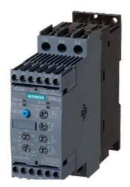
SIRIUS SOFT STARTER, S2, 45A, 22KW/400V, 40 DEGR., AC 200-480V, AC/DC 110-230V, SCREW TERMINALS
